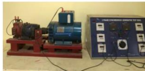
3Phase Synchronous Test ring
